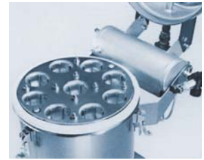
effective filter cleaning by means of compressed air counter-flow
