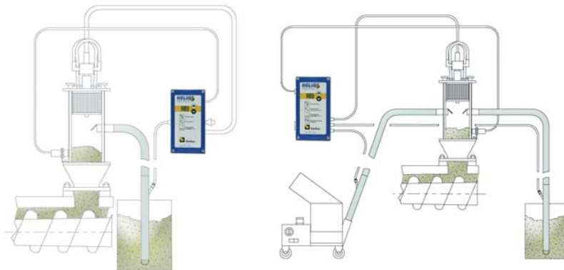
Mounted on an intermediate container or directly on feed zone.
