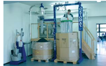
Refilling station with vacuum station
