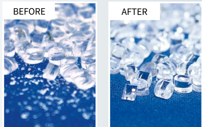
PMMA raw granules before and after dedusting.
